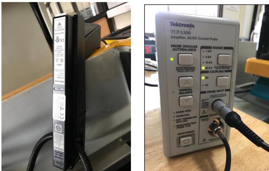
**Fig. 3.4** Current probe and current probe amplifier
