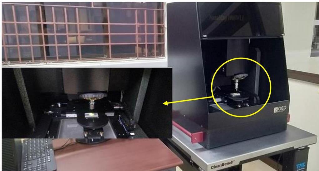
**Fig. 3.16** Non-contact 3D profilometer
