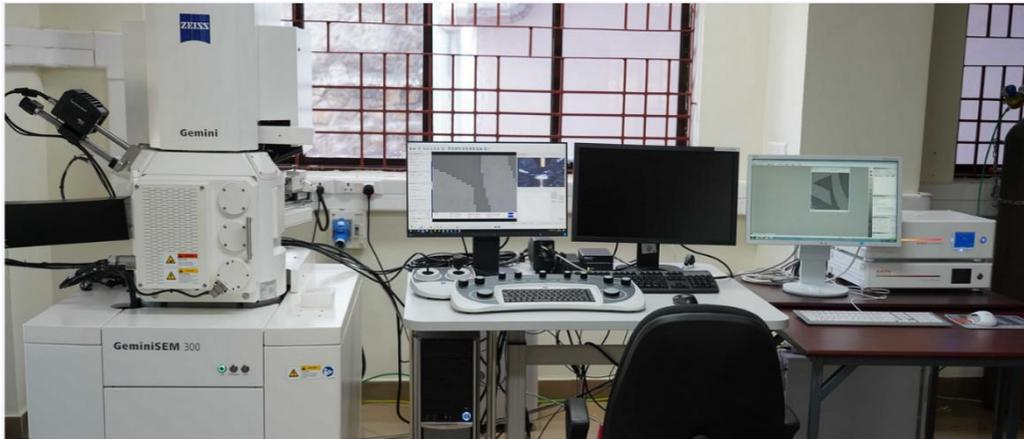
**Fig. 3.14** Field emission scanning electron microscope (FESEM) setup
