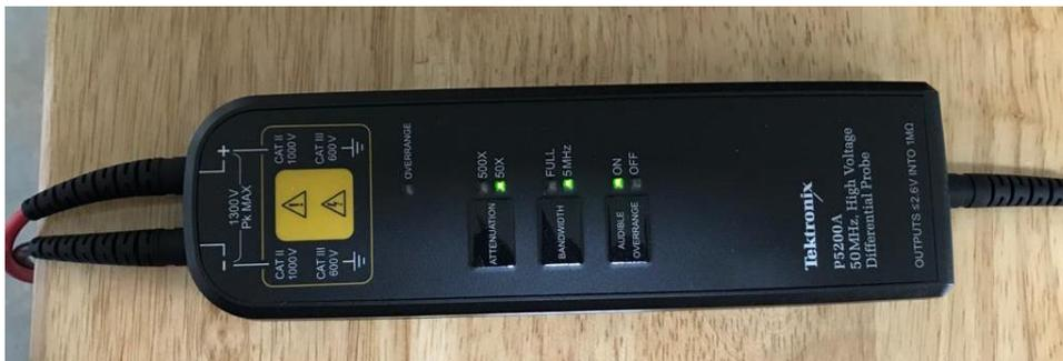
**Fig. 3.3** Differential probe
