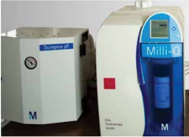
2. De-ionised water plant [1 number]: 60-liter-capacity, capable of producing Type II (at least 5 MΩ-cm resistivity ) & Type I (at least 18.2 MΩ-cm resistivity)
