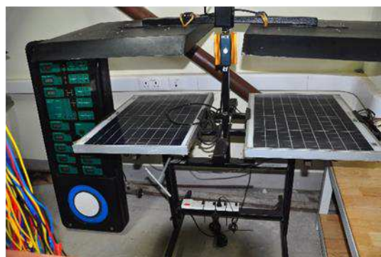
Power Systems Lab, Left: Alternator Fault Simulator wWith Grid Synchronization Facility, Right: Solar Photo Voltaic Array Simulator
