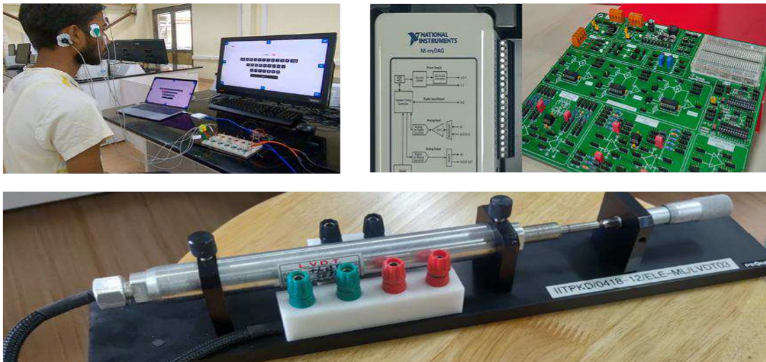
Measurements and Instrumentation Lab, In Clockwise Order from Top: Electro-oculogram EOG Data Acquisition, Analog Signal Conditioning (TI ASLK) and Data Acquisition (NI MyDAQ) and Linear Variable Differential Transformer (LVDT) setup
